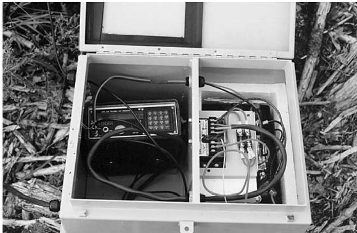
VHF receiver-datalogger that allowed recording of 24 h activity budgets. Photo by S. Côté.
