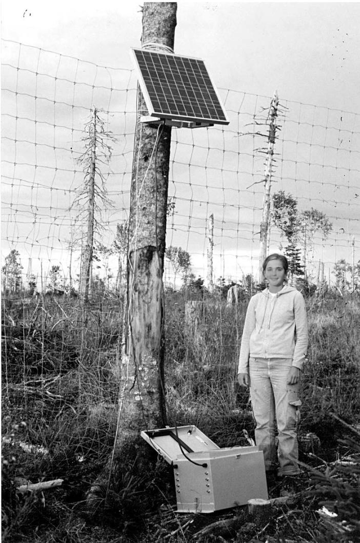
VHF receiver-datalogger connected to a multidirectional antenna and solar panel. Photo by S. Côté.
